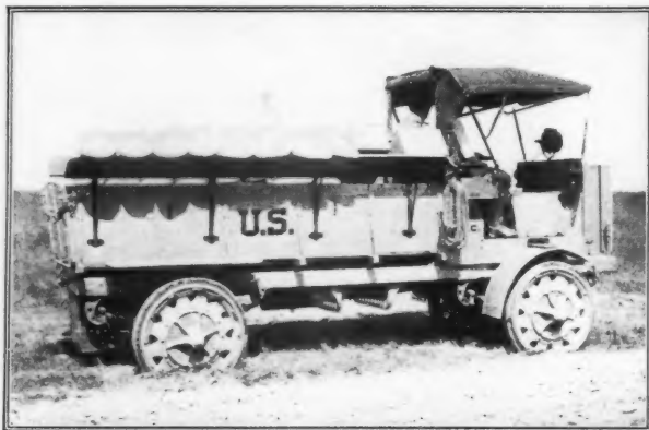
One of the trucks used in the Mexican punitive expedition—a Jeffery "Quad" which drives through all four wheels
